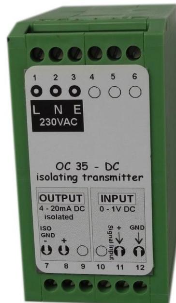
**OC35-DC** are transmitters for DC voltage or DC current. The input signal is converted into standardized output 4-20mA or 0-10V. The analogue outputs can be ordered isolated or non-isolated. The transmitters are supplied from the mains or from DC voltage.
