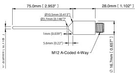
Weld burr may extend 1mm from colar to towards tip of probe
