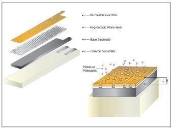
Michell ceramic metal-oxide moisture sensor tile layers
