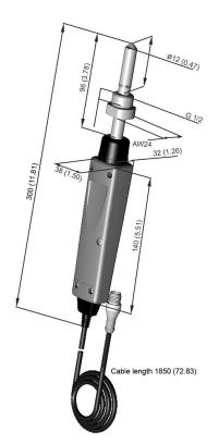
Probe dimensions in millimeters (inches)
